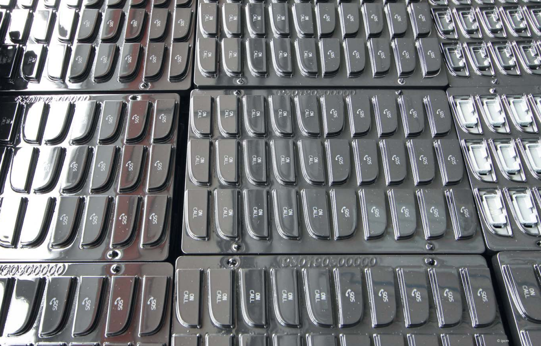
Some keys printed, laser engraved, and coated by Barnem Technologie Plastiche Srl.
